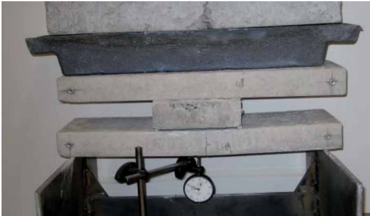
Set-up creep test Specimen with steel fibre concrete after 1600 days.
