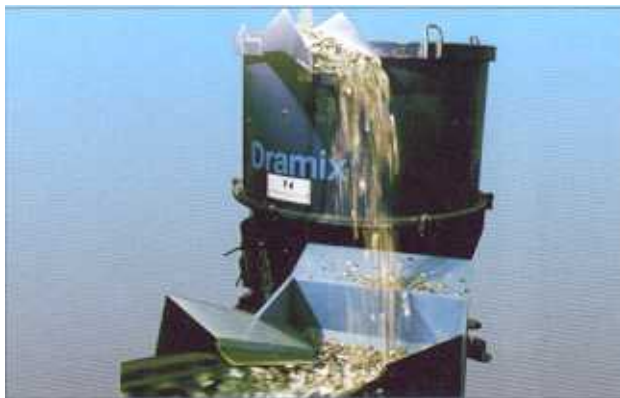
Automatic dosing and dispensing equipment.
