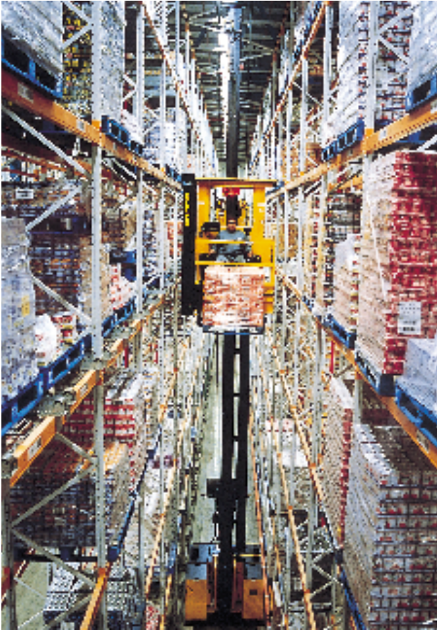
Superflat jointless warehouse floor. Discontinuous reinforcement makes a superflat floor easier to construct. As there are no joints a high tolerance is maintained over the whole area.
